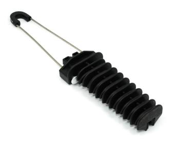
PA-2000 cable anchor clamp has been designed to ensure the rapid, simple and secure fastening of ADSS fibre optic aerial cables in a range of diameters from 10 to 15 mm. Anchor clamp consists of removable stainless cord, UV resistant plastic wedges and body. The automatic, conical tightening system provides no additional tools are necessary and considerably reduces installation time.
